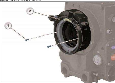
4. Remove the lens lock (1) from the PL mount. Keep all installed shims (if any) carefully in place (2):
