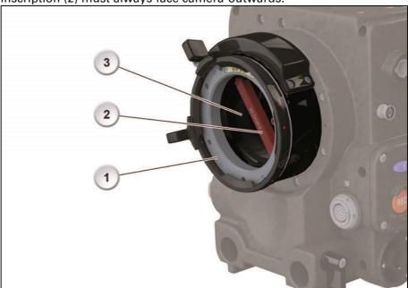
3. Untighten the reflex tube (2) with the wrench (1) and unscrew it with your fingers. Do not touch the sensitive sensor glass:
