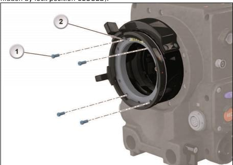
3. Turn the lens lock into position OPEN (2) to unhide and unscrew the other two torx screws (1):
