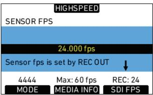
Figure 45: SENSOR FPS screen with linked sensor frame rate
