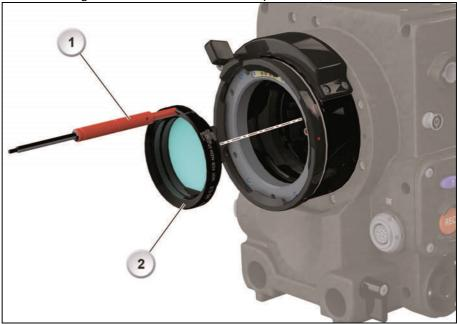
7. Place the next filter onto the bottom ring in the camera's PL mount. The Ground Glass/Frameglow tool has to be in the 12 o'clock position (1):
