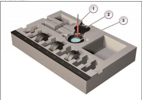
6. Make sure the next filter is clean (2) and the Ground Glass/Frameglow tool is in the 12 o'clock position (1):
