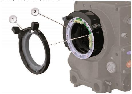
5. Accurately place the IFM Shim, with its inscription always facing camera-outwards (2), onto the PL mount. The shim's screw holes must line up exactly with the mount's thread holes and the index pin (3):
