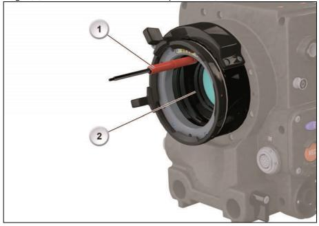
3. Pull the filter (2) from the bottom ring in the camera's PL mount. If the filter position is held by an IFM Empty Filter Frame (applies only to ALEXA XT), remove it likewise:
