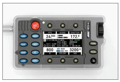
The camera can be remotely controlled with an RCU-4. This device mirrors the controls on the camera's right side. It is connected to the camera's Ethernet port. Power is supplied via the Ethernet cable.
