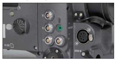
Figure 16: 24 V outputs (RS) and 12 V output
