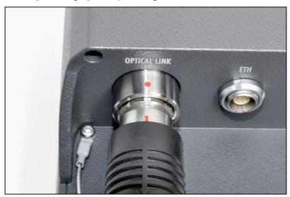
Figure 136: Correctly aligned fibre connectors
