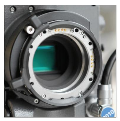
Figure 79: Lens adapter PL-Mount LA-PL-2 (with LDS)
