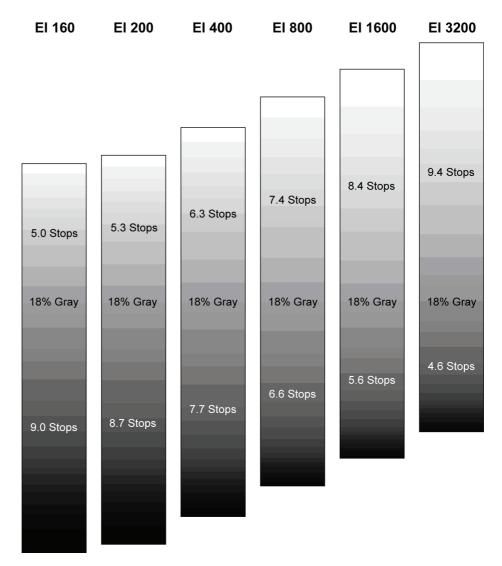
Figure 53: Graphical comparison of latitude at different exposure indexes
