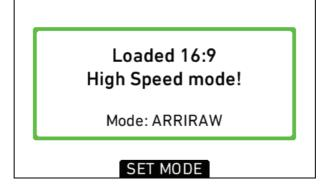
Note: Starting from 4:3 Normal Speed, the resulting High Speed mode differs depending on the currently selected recording mode: With ProRes recording selected, the ALEXA will go to 16:9 High Speed. With ARRIRAW recording selected, the ALEXA will go to 4:3 High Speed. Exiting High Speed mode will always return to 4:3 Normal Speed.
