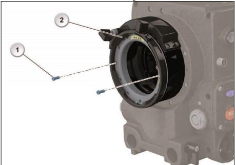
7. Turn the lens lock into Position CLOSED (2) and fasten the other four torx screws hand-tight (1). Check if all screws and the shim fit correctly:
