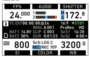
Note: The use of the internal ND filter has no influence on the EI rating of the camera. When measuring exposure with a light meter, take into account the light loss of 4 1/3 stops generated by the ND filter.
