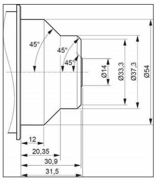
Figure 137: Allowed lens dimensions with in-camera filters
