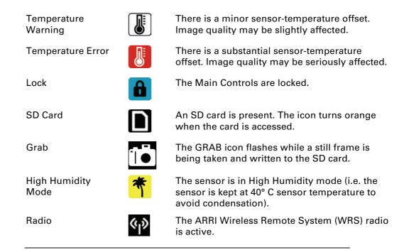
Note: A sensor temperature warning or error after boot-up is normal as the sensor takes a few seconds to reach its preset temperature.
