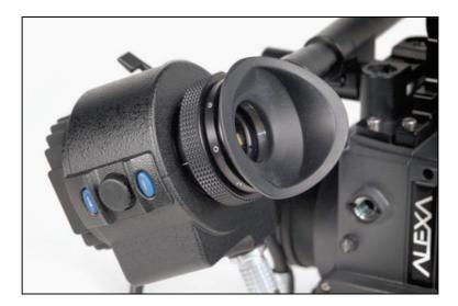
The electronic viewfinder EVF-1 employs a liquid crystal on silicon (LCOS) imaging device with a temperature-stabilized LED light source to provide a bright, accurate view of the sensor image in all operating conditions. Each EVF-1 is calibrated to precisely match the image on the ALEXA's HD outputs.
