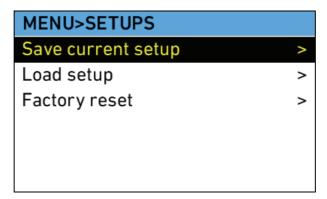
A user setup is a profile of the current settings on the ALEXA that can be saved to the SD card. User setups can be given custom names, saved to the SD card and loaded onto multiple ALEXAs.
