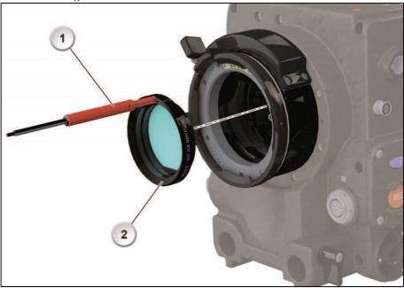
4. Clean the removed filter and stow it properly in its individual box and the storage case. If the filter position was held by an IFM Empty Filter Frame, store it likewise (in case the camera is no longer shimmed for IFM-1 in the future)
