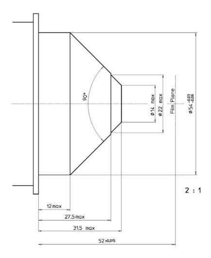
Figure 102: Allowed lens dimensions with mirror shutter
