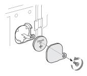
Insert a new backup battery (CR2032) with the + symbol on the battery facing outside.
