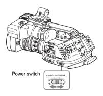
To operate in Camera mode, turn the power on by setting the power switch to the CAMERA position.
