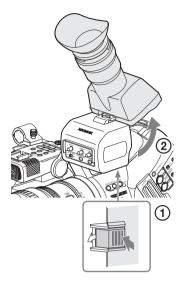
Normally use it in the locked position. Although you can open it farther from the lock position, once return it to the closed position to lock it at the 120-degree position again.
