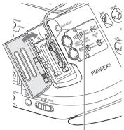
Pass through the cable guide slot.
