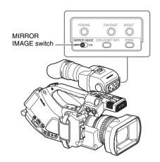
When the camcorder is in Media mode, the picture is also inverted both vertically and horizontally. In Camera mode, the picture is inverted only vertically, while it is also inverted horizontally for Rec Review (page 72).
