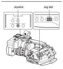
1 Tilt the joystick or turn the jog dial to set the cursor to "Date/Time" then press the joystick or dial.
