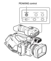
The color of the contours can be set with "Peaking" (page 121) of the VF SET menu. Turning the control back to its left stop position deactivates the peaking function.
