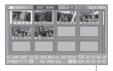
The detailed information of the clip is displayed at the bottom of the screen.
