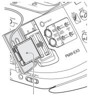
Insert so that the cable extends upward.
