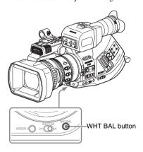
During adjustment, an in-progress message is displayed on the screen. When the adjustment is completed successfully, the message changes to a completion message, and the obtained color temperature is displayed.
